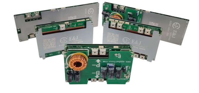
The EJ Series Smart BMS is compatible with ternary lithium, lithium iron phosphate, and lithium titanate battery packs ranging from 4S to 24S configurations.
