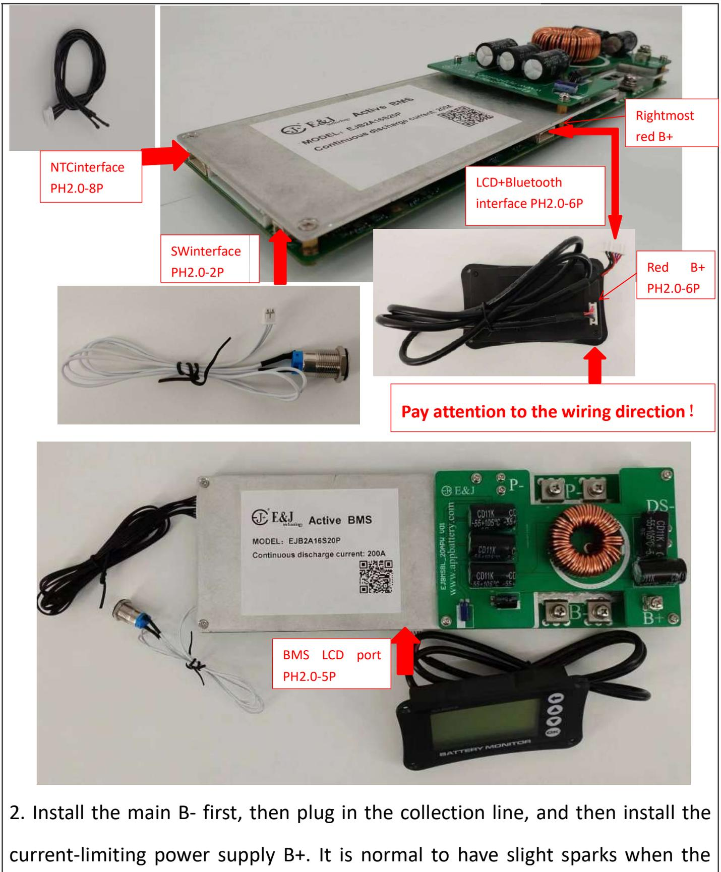
current-limiting plate capacitor is charged at the moment of power-on.
