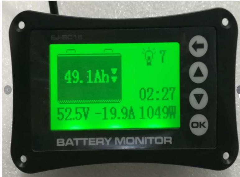
6.3 Press and hold the OK button on the LCD screen to display the single cell voltage of the battery pack, press ▼ ▲ to page up and down to view
