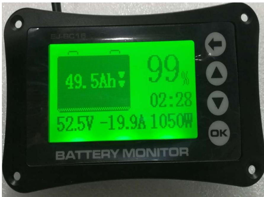
6.2 press ▼ ▲ button to adjust the LCD screen display brightness, press and hold ← button to turn the LCD screen light on and off
